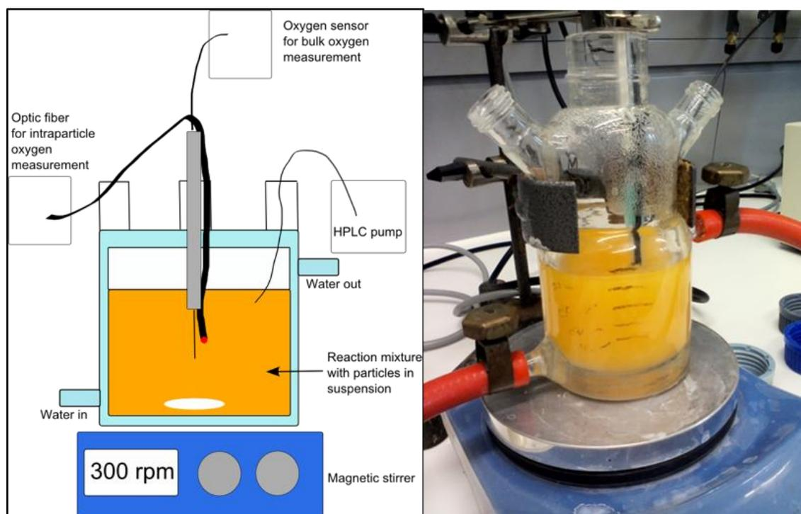
**Figure 5.** Set-up for scaled-up reactor for running a conversion of D-Met with a labeled (orange) coimmobilizate of *Z<sub>basic2</sub>\_Tv\_DAAO* and *Z<sub>basic2</sub>\_BP\_KatA*.
