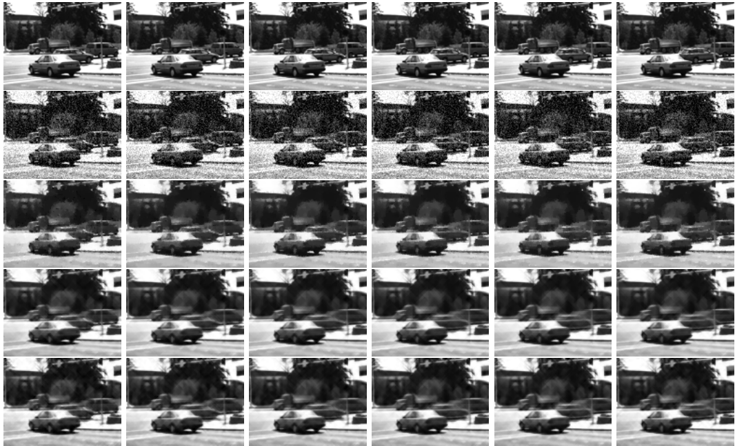
Figure 4.18.: First row: Ground truth from " http://vision.middlebury.edu/flow/data/ ". File: Dumptruck. Second row: Given data, with added Gaussian noise with a standard deviation of \sigma = 0.1 . PSNR = 20 dB Third row: Denoising using TV-regularisation. PSNR = 25.47 dB Fourth row: Denoising using TVX 0 . PSNR = 25.64 dB Fifth row: Denoising using TVX 1 . PSNR = 25.86 dB
