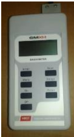
Figure 6: Gaussmeter GM 08 for 3D scanning and direct measurements
