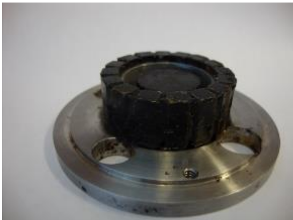
Figure 9: Configuration of permanent magnets on a ferromagnetic steel plate in the cathode.
