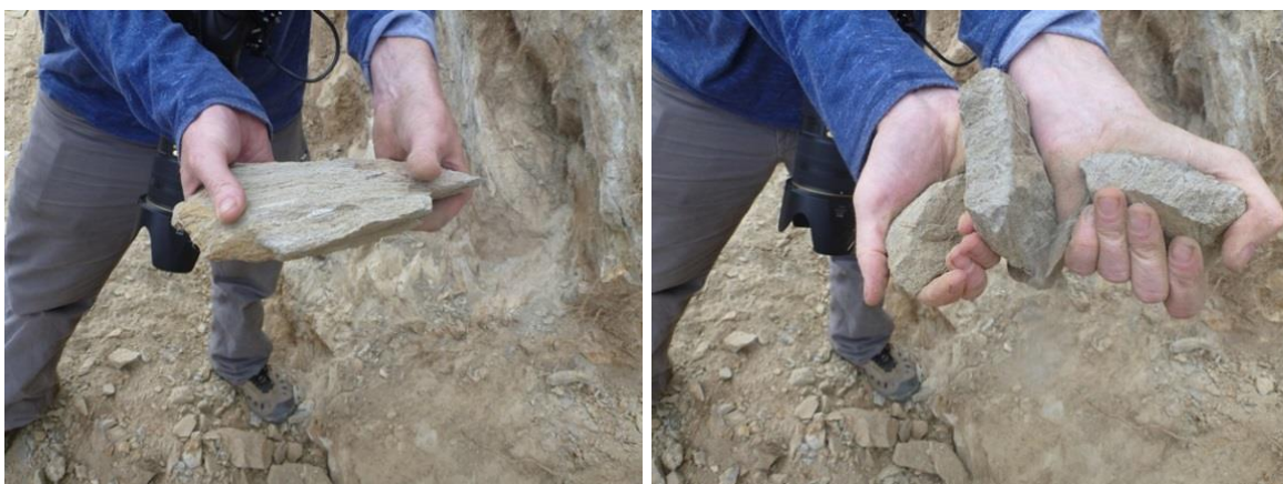
Figure 66 Some of the viewed outcrops along the road exhibited highly weathered rocks (mostly Gneiss), which are described as friable due to their preserved texture but high breakability (© Ziselsberger)
