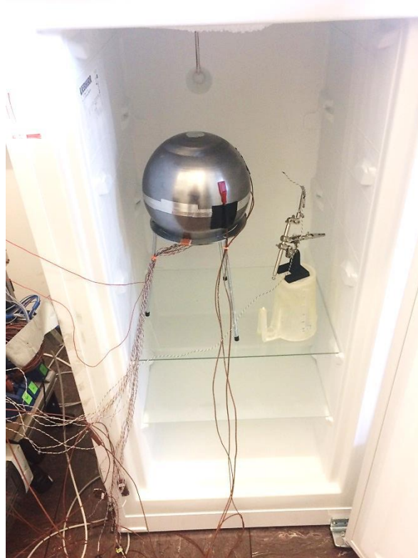
Figure 40 Filled sphere put into the refrigerator and the additional thermocouple to measure the ambient temperature
