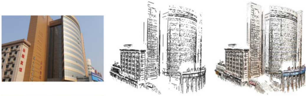
Figure 2.17: Illustrations taken from [26]. Left: An example image of their Press Building dataset (100 images, 2128 \times 1416 px). Middle: Obtained 3D line model. Right: The 3D line model and the dense PMVS [49] point-cloud combined.
