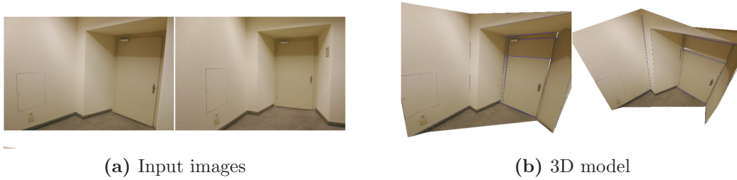
Figure 2.7: Illustrations taken from [16]. (a) Two uncalibrated input images of an untextured indoor scene. (b) The resulting piecewise planar 3D model obtained from matched line segments, and automatically detected planar image regions using line junctions.
