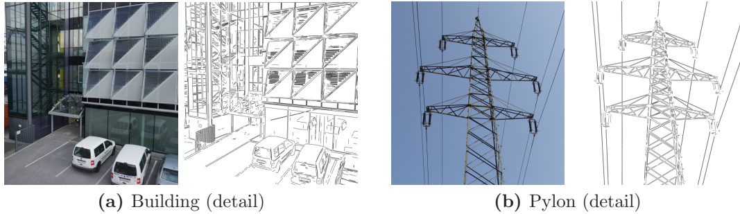
Figure 3.5: Line segment detection using the LSD algorithm [51]. (a) Example image from the Building sequence (3801 segments). (b) Example image from the Pylon sequence (6875 segments).
