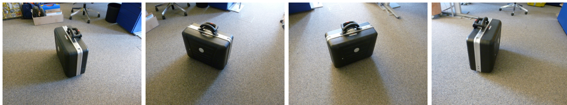
Figure 5.1: An example of an unsuitable image set for SfM reconstruction, as taken by a non-expert user. As we can see, the relative camera motion between consecutive images is too large for reliable feature matching.
