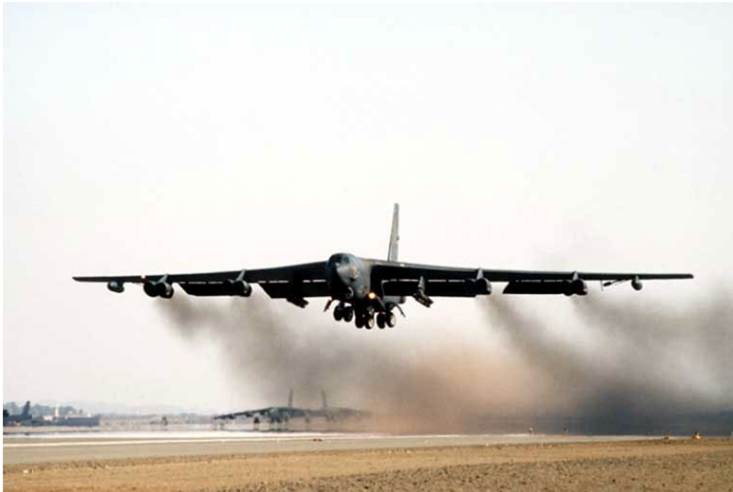
Figure 4: B 52 at takeoff with water injection. Soot plumes can be seen behind the engines (image courtesy: US Air Force).
