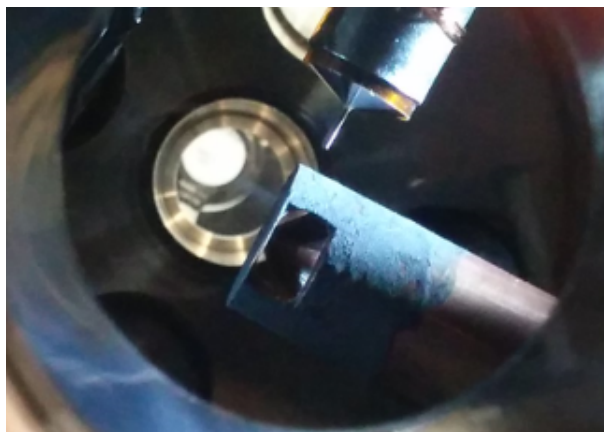
Figure 2.9: Picture of the repeller with the soft iron truncated cone and the tip of the oven, which is used to evaporate solid specimens.
