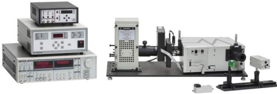
**Figure 3.5:** EQE measurement system<sup>[12]</sup>
