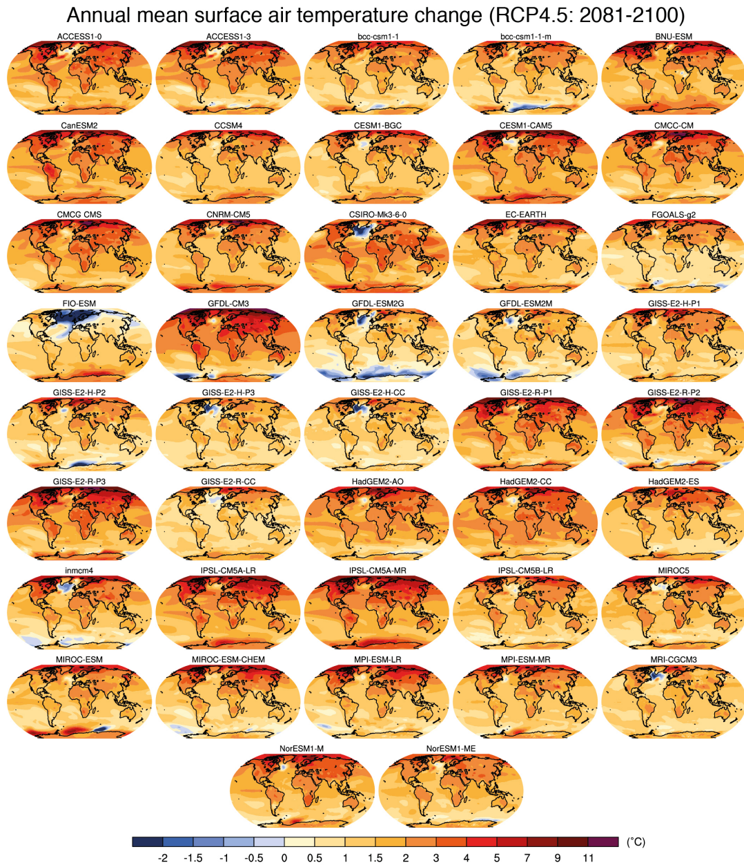
Figure 2.3: Projected CMIP5 temperature climate changes from 1981-2000 to 2081-2100, as presented in the fifth assessment IPCC report. The individual GCMs are driven with the RCP4.5 external forcing. Source: Collins, Knutti et al. 2013.
