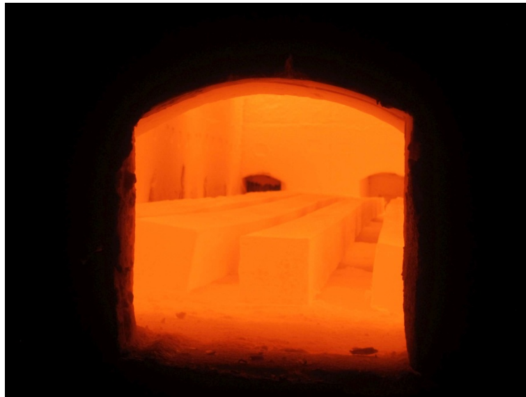
Fig. 28. Steel billets on the stationary hearths right before discharging (discharging door in the background).
