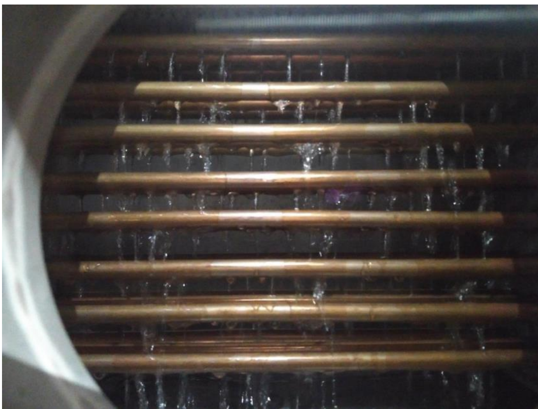
Figure 53: Wetting of the tubes caused by the falling film
