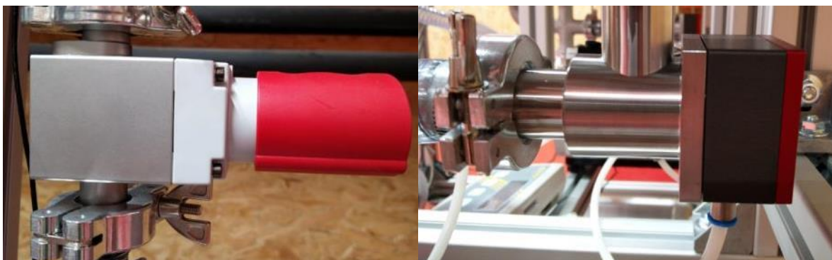
Figure 26: Manuel valve on the left, pneumatic valve on the right
