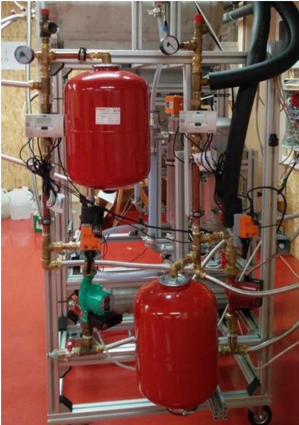
Figure 66: Hot and cold water circuit, on the right side connected to the test rig, on the left side connected to the labor
