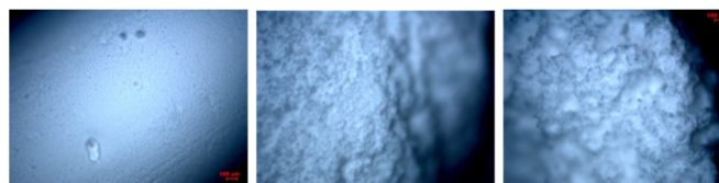
Fig. 21: Outer structure of dried IMEO monoliths (type A). From left to right: low - middle - medium porogen content, (bright field mode)
