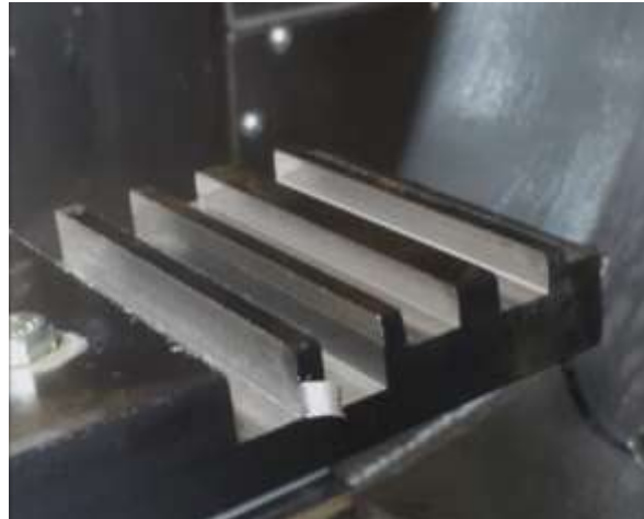
Figure 59. Milled workpiece with different depths of cut, Source: Own contribution
