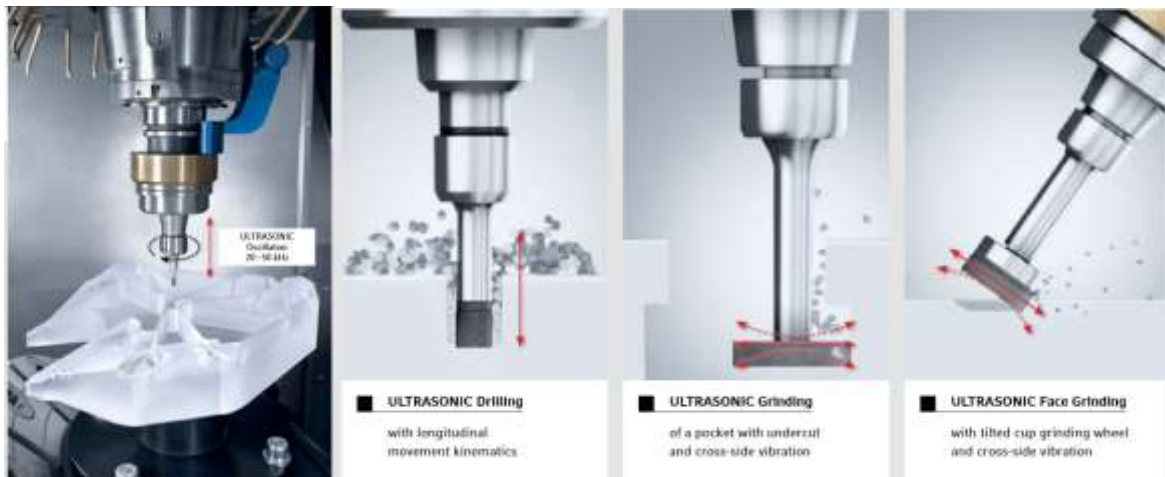
Figure 22. Machining Strategies for ULTRASONIC 30 linear, Source: DMG MORI, 2016
