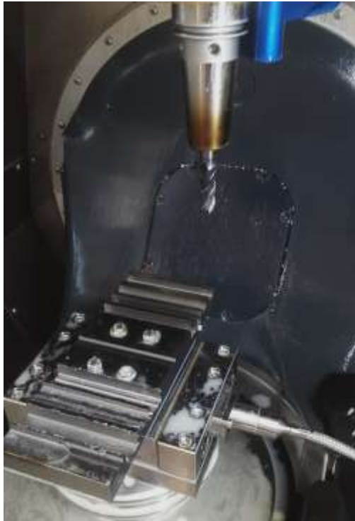
Figure 59. Milled workpiece with different depths of cut, Source: Own contribution
