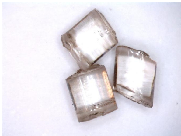
Figure 53: PC pellet impregnated by using \text{Cu}(\text{HDz})_2 in \text{scCO}_2 -ethanol mixture
