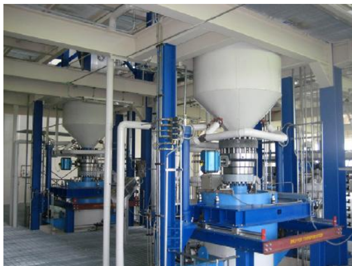
Figure 4: Industrial scale antisolvent process for powderous dried lecithin production, Uhde GmbH, Hagen, Germany [38]
