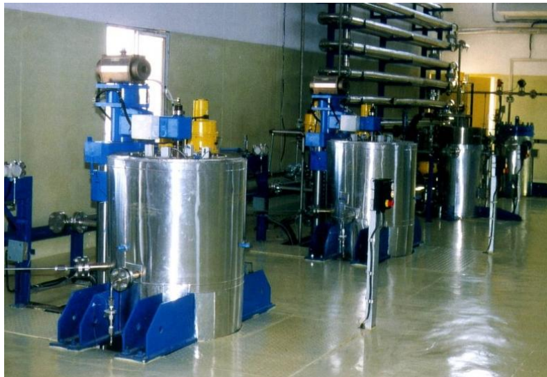
Figure 3: Supercritical extraction plant (600 liters, 550 bar) for spices and herbs, India [15]
