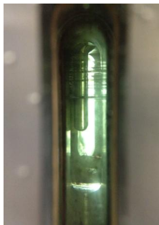
Figure 19: Dithizone dissolves in scCO_2 with light green color at 150 bar and 45 °C
