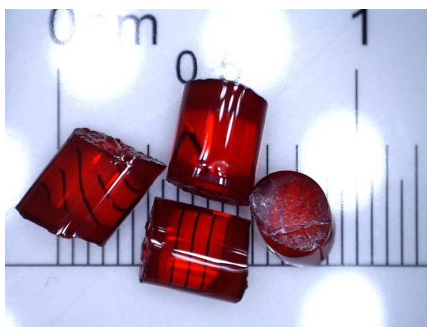
Figure 34: PC pellets impregnated with DR13 at 200 bar, 50°C for 3 hours of sorption time
