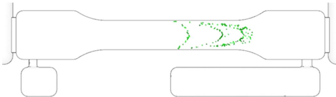
(c) Large overflow volume on the right side: The weld face is washed-out.
