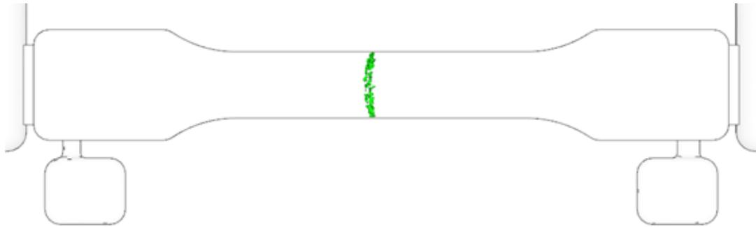
(a) Small overflow volume on both sides. A sharp weld face is obtained.
