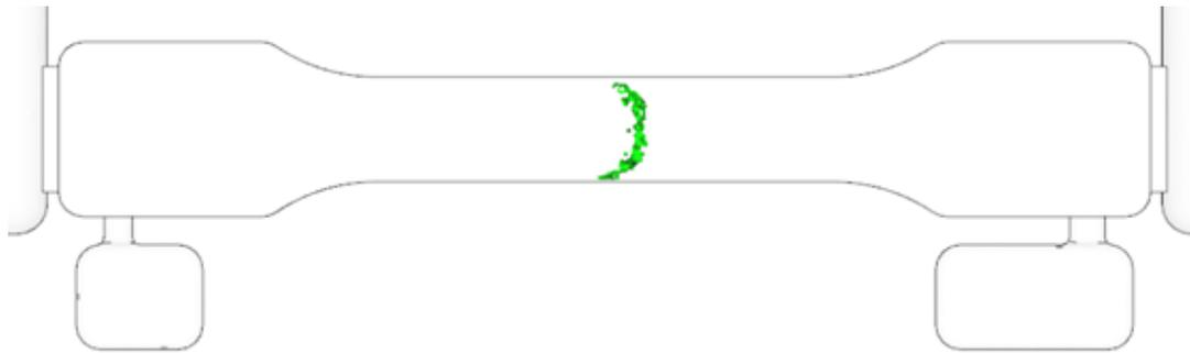
(b) Medium overflow volume on the right side: The weld face is distorted.
