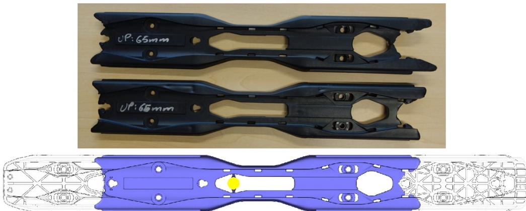
Figure 3.29.: Comparison of short shots made with PA6 GF45 (upper part) and unfilled PA6 (lower part). The simulated flow front was obtained using PA6 GF45.
