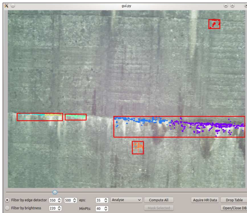
Figure B-1: GUI for identifying and registering defects
