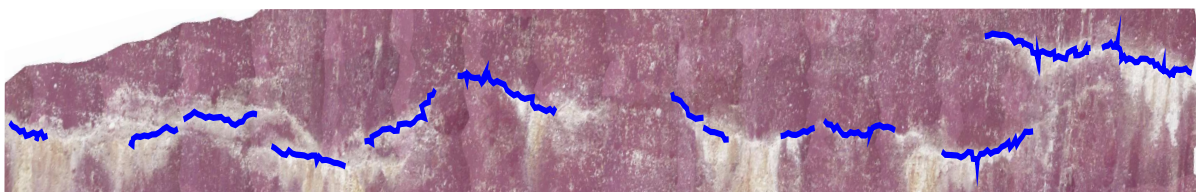
(c) Orthophoto overlaid with extracted crack polylines
