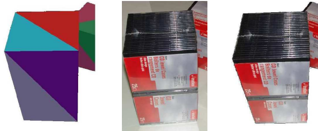
Figure 3-8: Example of a simple texture mapping (Hanusch, 2010, p. 5)
