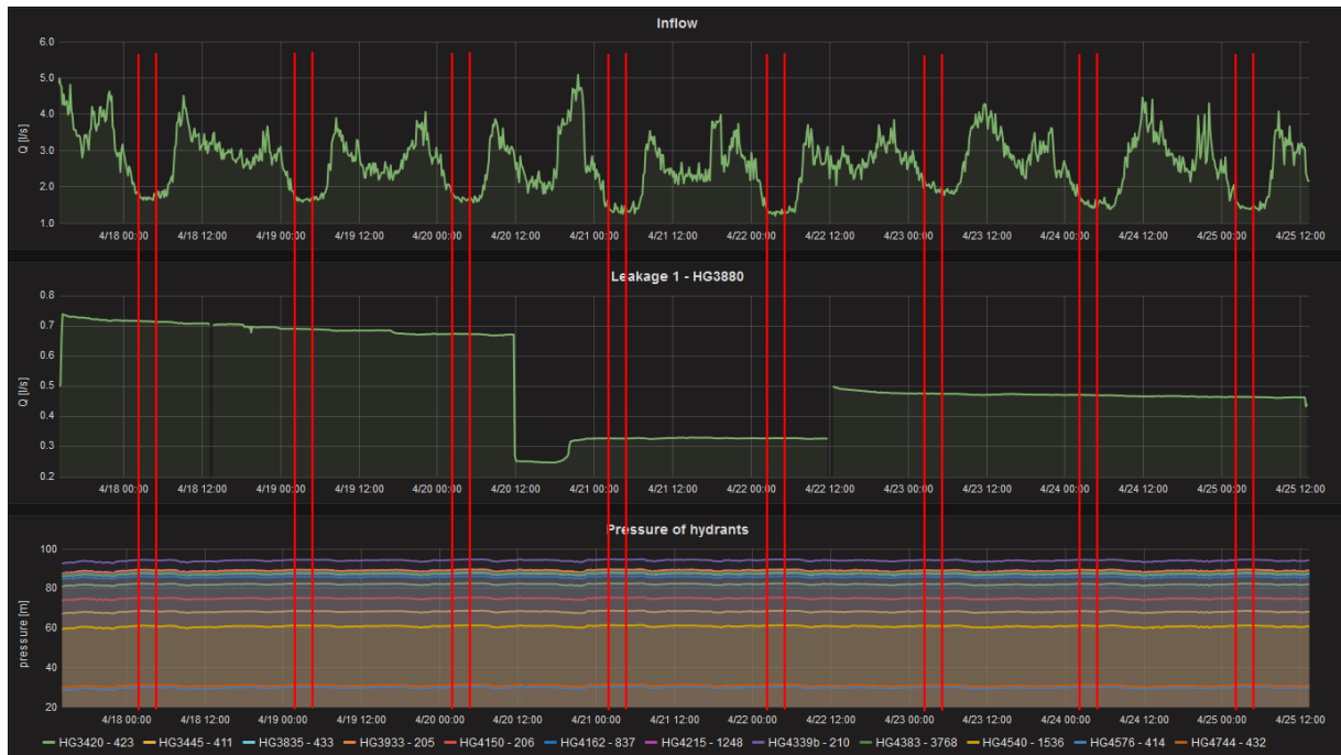
Figure 3.18: Evaluation of the leak measurement at hydrant HG3880
