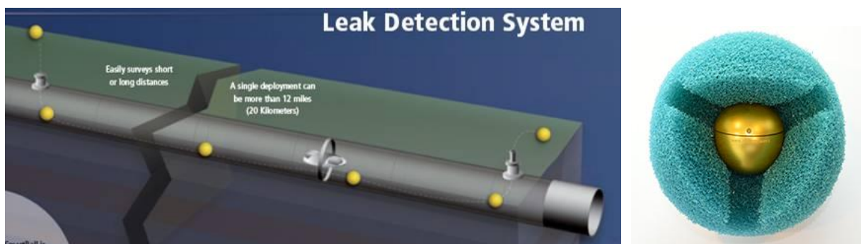
Figure 1.10: Smart Ball® Injection Process (Pure Technologies)
