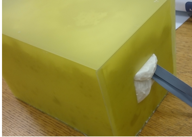
Figure 54: The devices were embedded in polyurethane foam to exclude the effect of natural convection.
