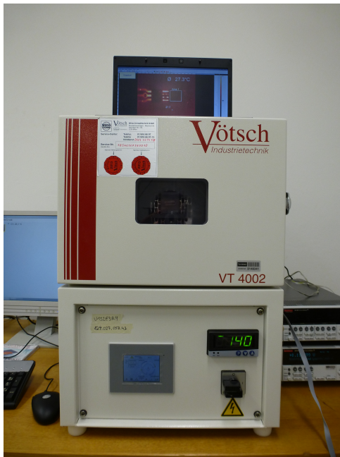
Figure 14: Vötsch ® VT 4002 climate chamber used to control ambiance conditions.
