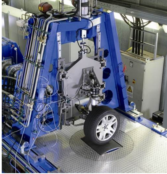
Figure 3.2: Test bench set up at Institute of Automotive Engineering, TU Graz[9]
