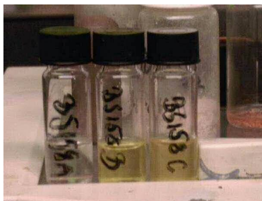
Figure 5.20 Reaction solutions of \text{Dipp}_2\text{SnH}_2 with (\text{CH}_3\text{Si})_2\text{NH} (HMDS-H, left), (\text{CH}_3\text{Si})_2\text{NLi} (HMDS-Li, middle) and \text{Et}_2\text{NLi} (right).
