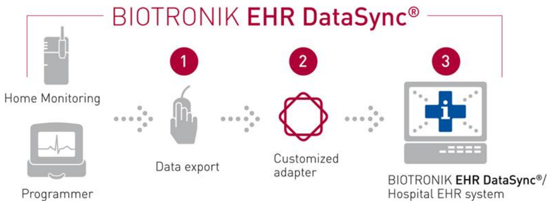
Figure 15: Data flow of Biotronik EHR DataSync®. The acquired data are exported from the home monitoring system or programmer (1). Then they are converted with the Biotronik Adapter (2) and imported in the EHR system of the hospital (3) [54].
