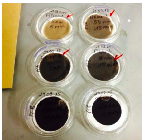
Figure 36: Image of the quartz tissue samples with different loadings of carbon nanoparticles. There are noticeable changes in the degree of black between the samples. This is presumably due to the different nanoparticle dimensions as well as different carbon concentrations.
