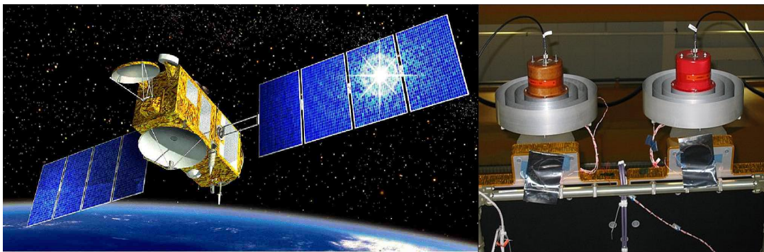
Figure 3.13: Illustration of the Jason 2/OSTM satellite in orbit (left) and GPS antennas with choke rings for POD (right). ©NASA
