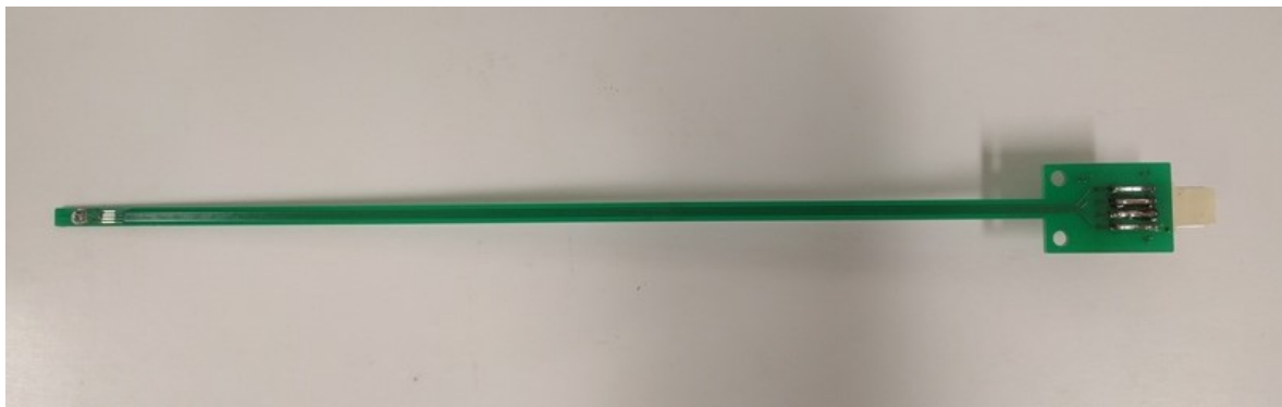
Figure 2.6: Image of the sample holder where the devices were bonded on. The device is situated on the end thin tail at the left side of the image.
