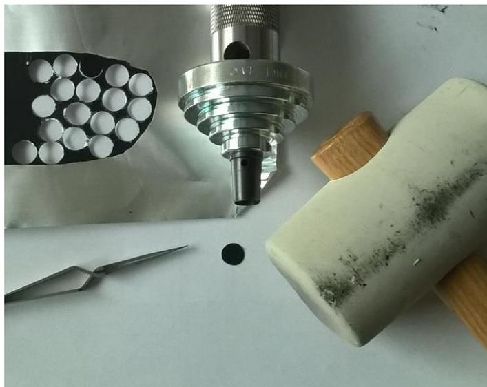
*Figure 30 Fabrication of the electrode (10 mm) by stamping the doctor bladed, activated cellulose on the aluminum carrier.*
