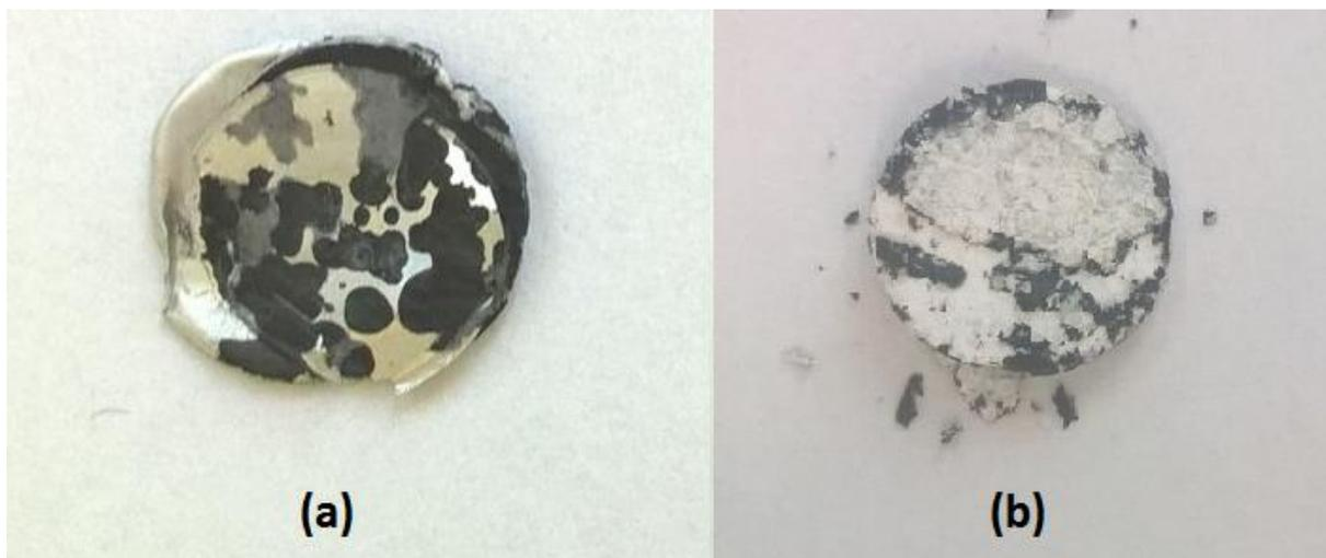
Figure 39 Images of electrodes after electrochemical characterization. (a) is with an alkaline as electrolyte (KOH), whereas (b) is measured with  $H_2SO_4$ .
