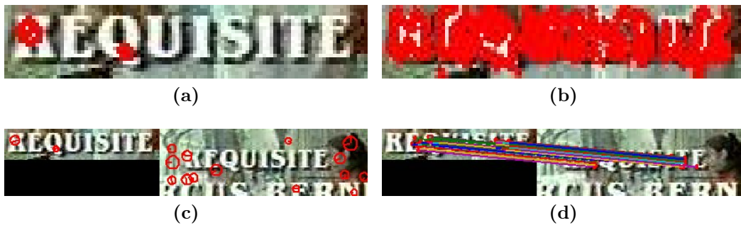
Figure 3.2: SWT-SIFT scheme by Phan et al. [68]: They compute SIFT [46] descriptors at each pixel of the text’s edges obtained by SWT . At the top the comparison of the amount of extracted features using native SIFT (a) and SWT-SIFT (b) is illustrated. At the bottom the NN matching of SIFT (c) and SWT-SIFT (d) is compared. Images taken from [68].
