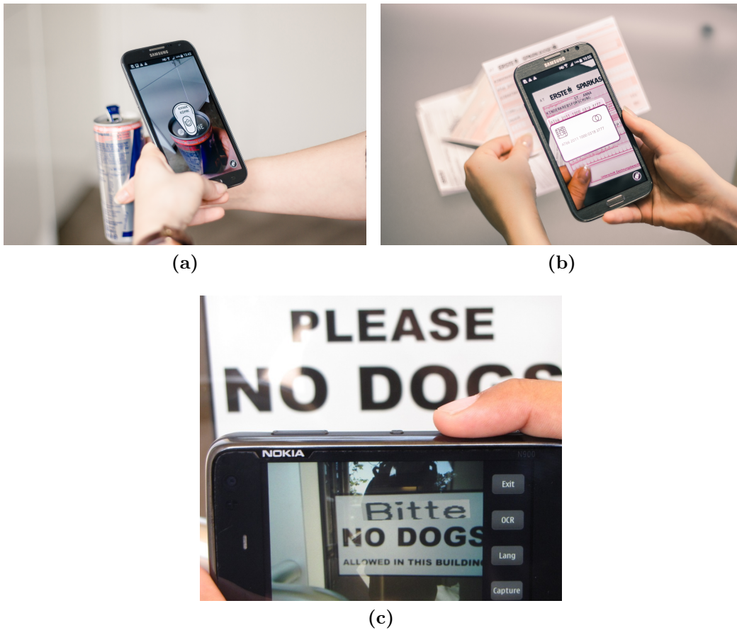
Figure 1.1: Several applications of text recognition on mobile phones. In (a) a winning code on a can lid is scanned, image (b) illustrated the scan of an International Bank Account Number (IBAN) to speed up a transaction process and in (c) scene text is recognized, translated and overlaid in the display. Image taken from web source 1 and [16].
