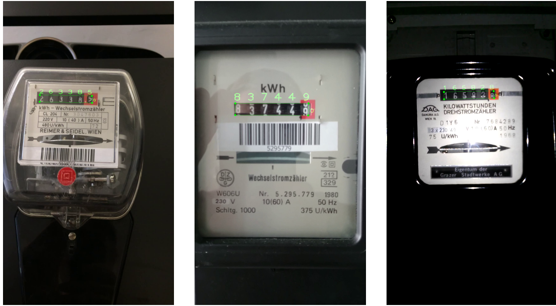
Figure 5.1: Exemplary frames of the evaluation datasets showing different types of energy meters and ground truth annotation. The digits of the meter readings are almost the only bright text on dark background. Reflections due to the front glass and the shiny surfaces, especially in combination with a camera phones flash light can mitigate the Optical Character Recognition (OCR) results.
