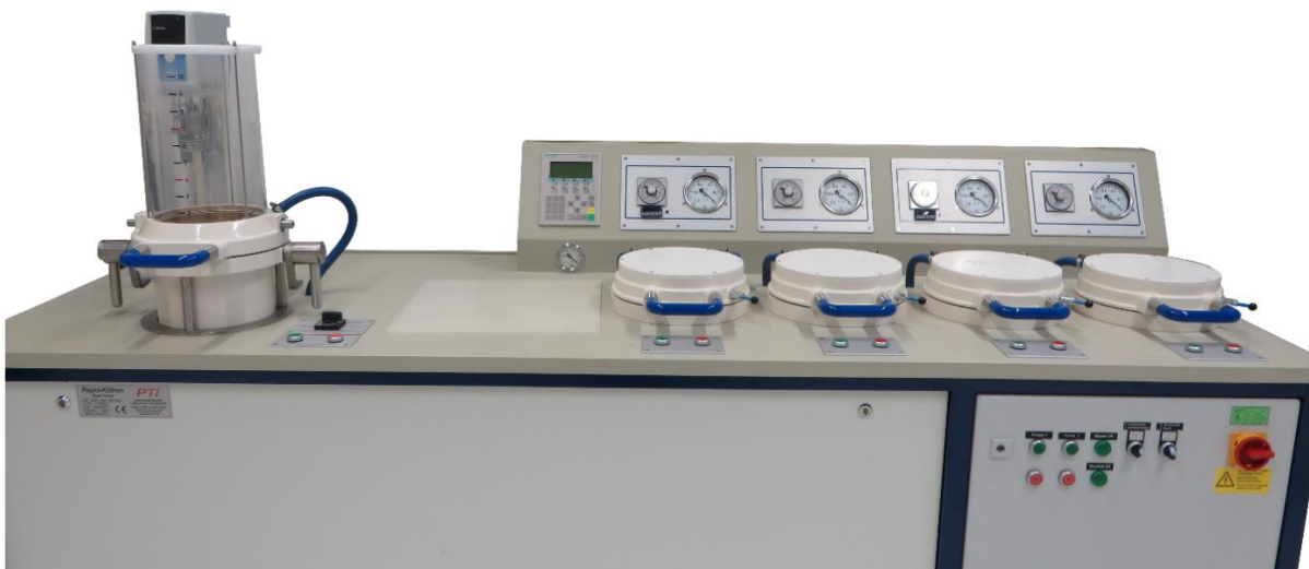
Fig. 4 Handsheet unit equipped with a white water recirculation system
