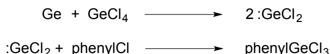
Figure 15. Preparation of phenylGeCl 3 via reaction of germanium metal and germanium tetrachloride and subsequent reaction of the dichlorogermylene with phenylchloride. 44
