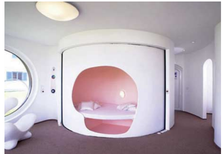
FIG. 104 The rotating cylinder inside the house contains bedroom, kitchen and bathroom [source: www.hanse-haus.de].
