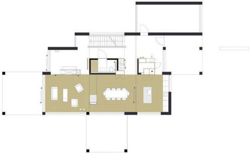
FIG. 92 The floor plan allows in three layers and with movable partition walls allows flexibility in the use. FIG. 93 [source: www.livingathome.de ].
