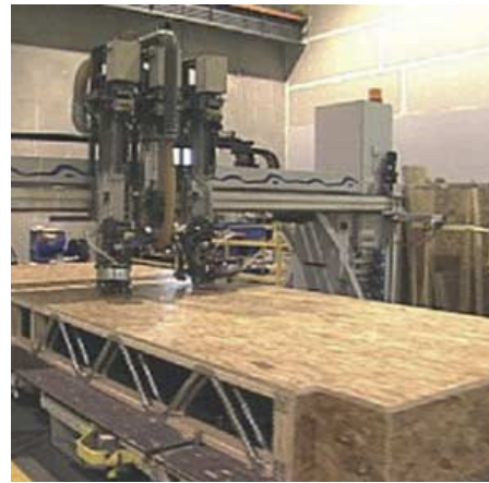
FIG. 95 Structural insulated panels in combination with steel are used to build the homes. [source: www.pulte.com]
