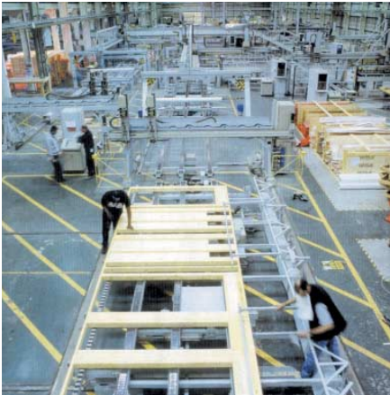
FIG. 96 The Space4 factory in Birmingham is producing timber-frame houses for the British market. (source: www.space4.com )
