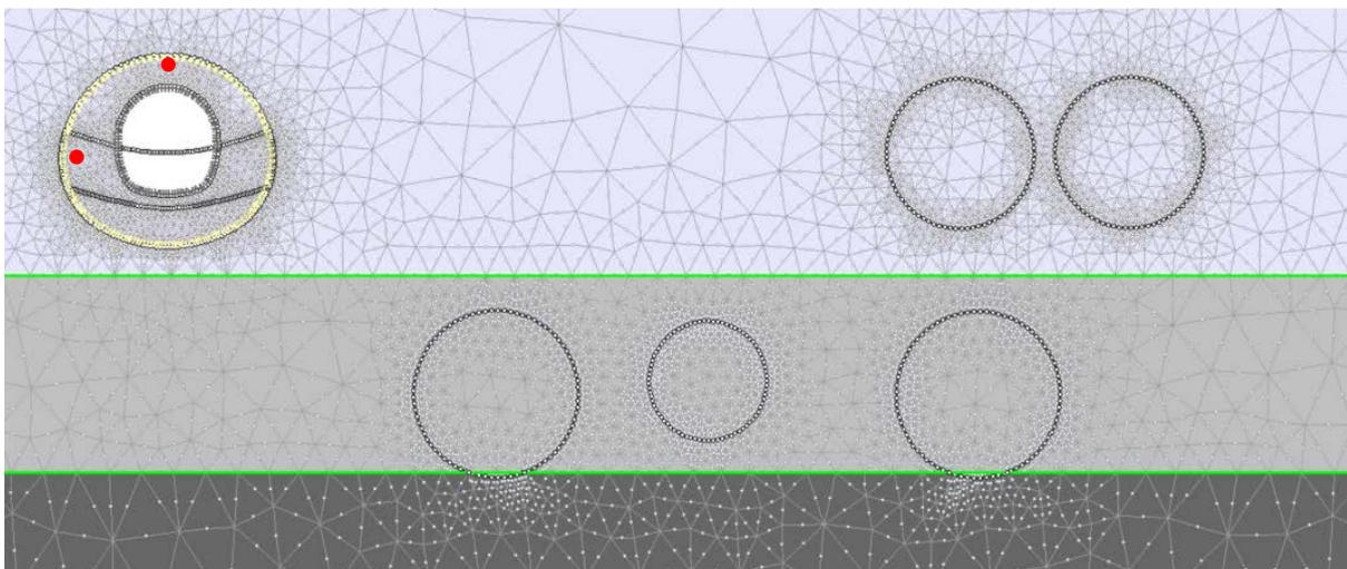
Figure 37: Position of measurement targets in platform tunnel
