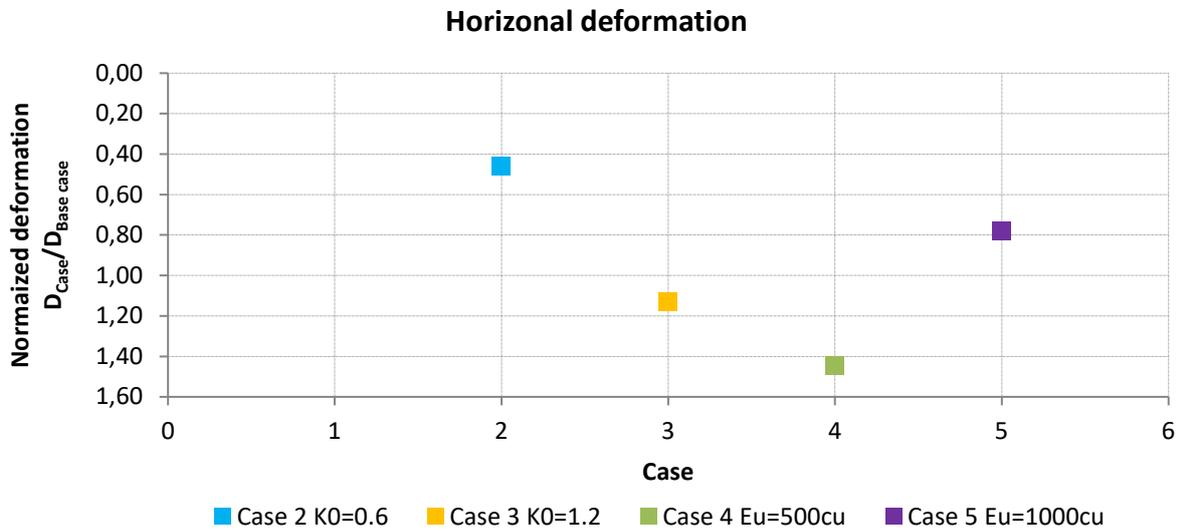
Figure 44: Normalized horizontal deformations (sidewall) of different cases
