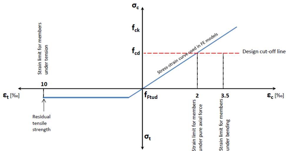
Figure 11: Stress-strain curve for steel fibre reinforced concrete (DSP, 2015)
