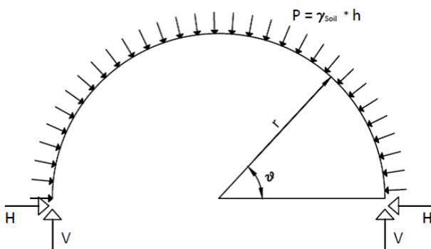
Figure 28: Lining stress system sketch
