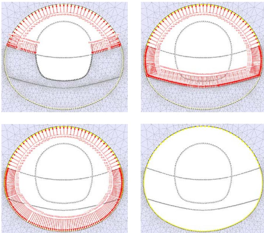
Figure 51: Excavation sequence platform tunnel convergence-confinement method
