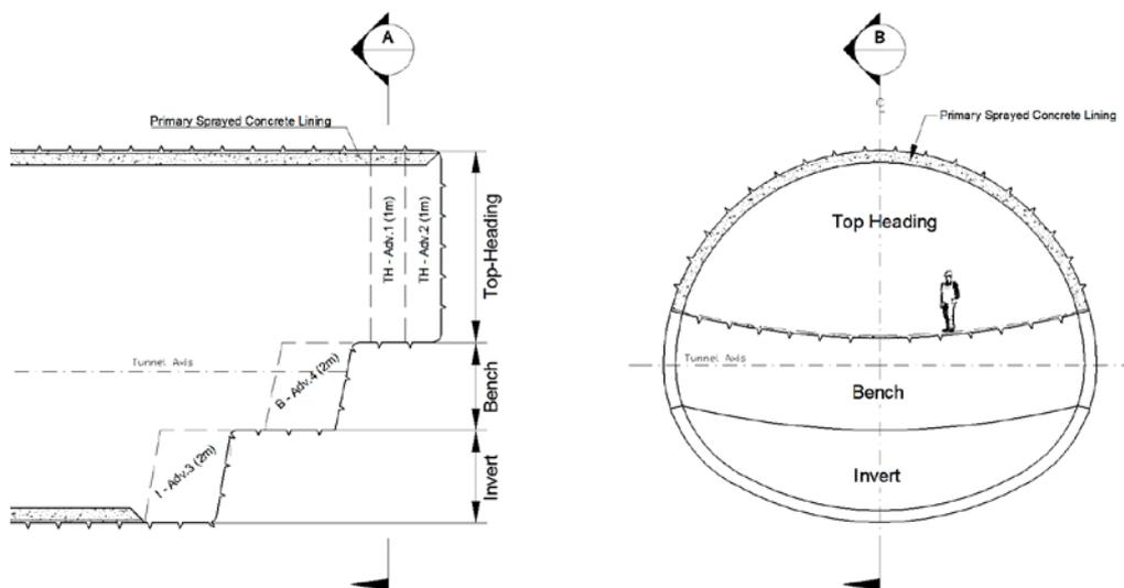
Figure 3: Excavation sequence top heading – bench – invert (DSP, 2016)
