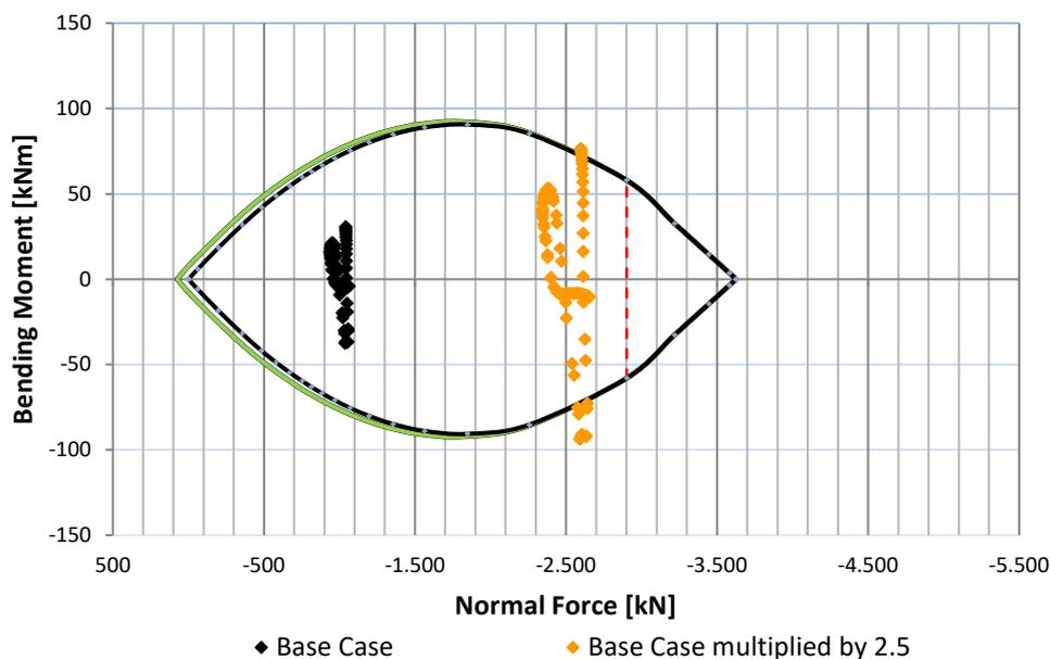
Figure 47: Bending moment vs. normal forces – base case multiplied by 2.5
