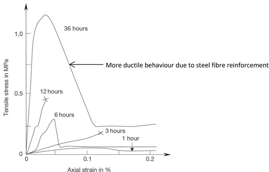
Figure 12: Tension behaviour at different ages (Euram, 1998)
