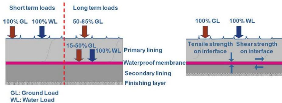
Figure 6: Load conditions for double shell and composite shell tunnel lining (Su, 2013)
