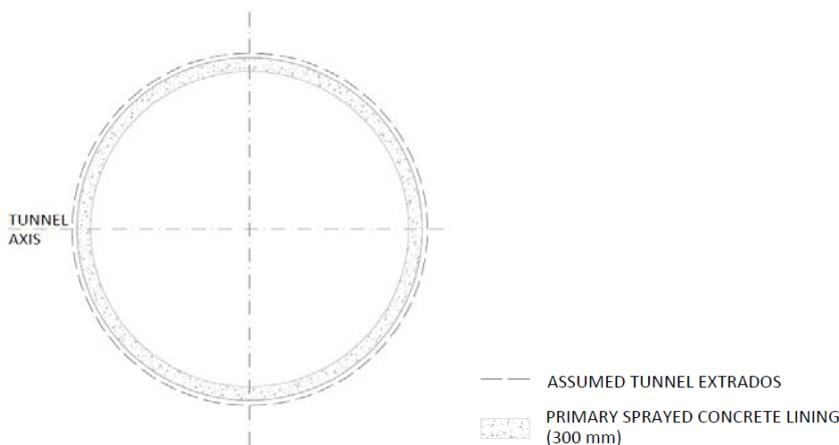
Figure 27: Used profile shape for calculation
