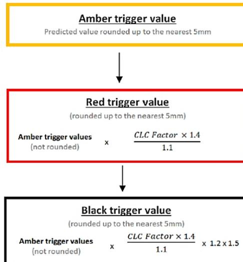
Figure 25: Determination of trigger values flowchart (Nasekhian, 2016)
