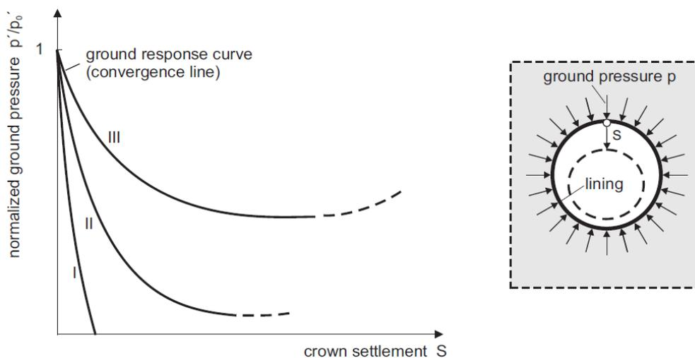
Figure 7: Ground response curves for different ground types after Pacher (1964)
