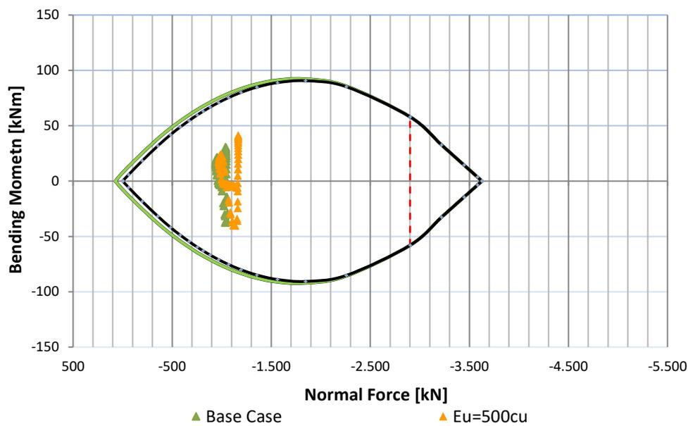
Figure 46: Bending moment vs. normal forces – base case vs. worst case
