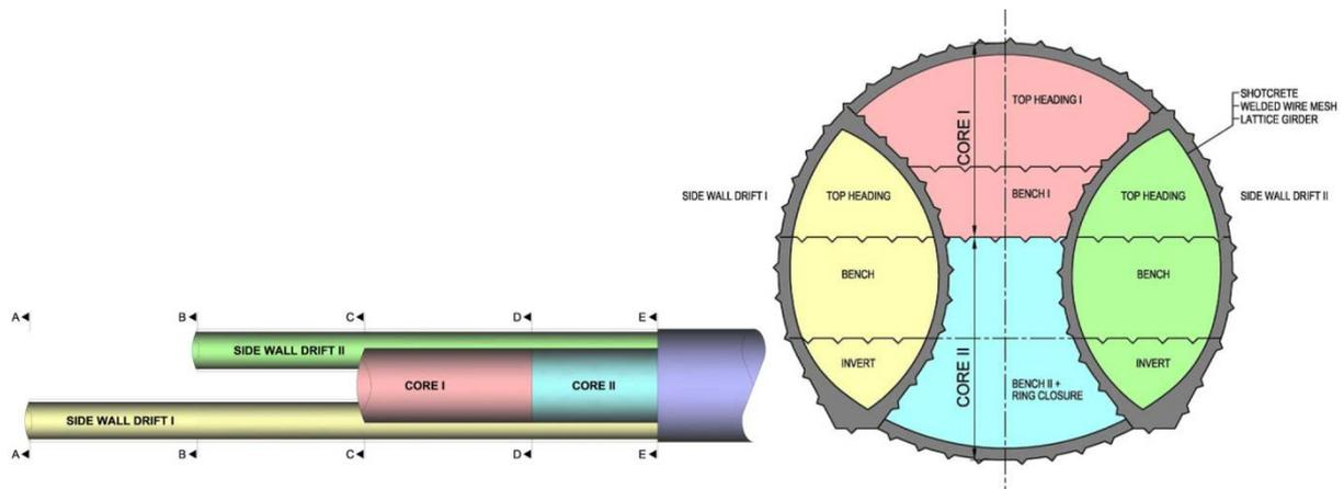
Figure 4: Side wall drift excavation method (The Austrian Practice of Conventional Tunnelling, 2009)
