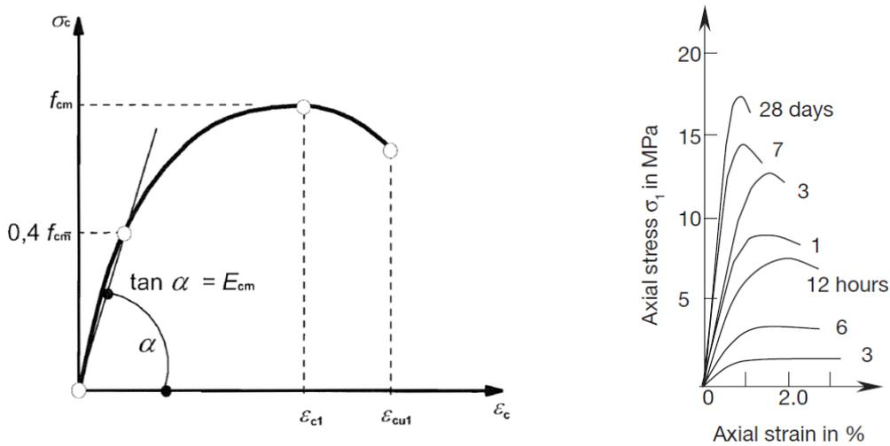
Figure 10: Stress strain relation (EC 2) & sprayed concrete of different age (Thomas, 2009)
