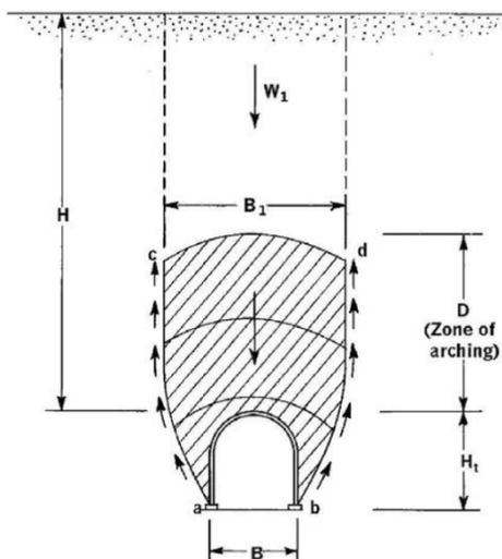
Figure 5: Loading on the tunnel lining (Terzaghi, 1946)
