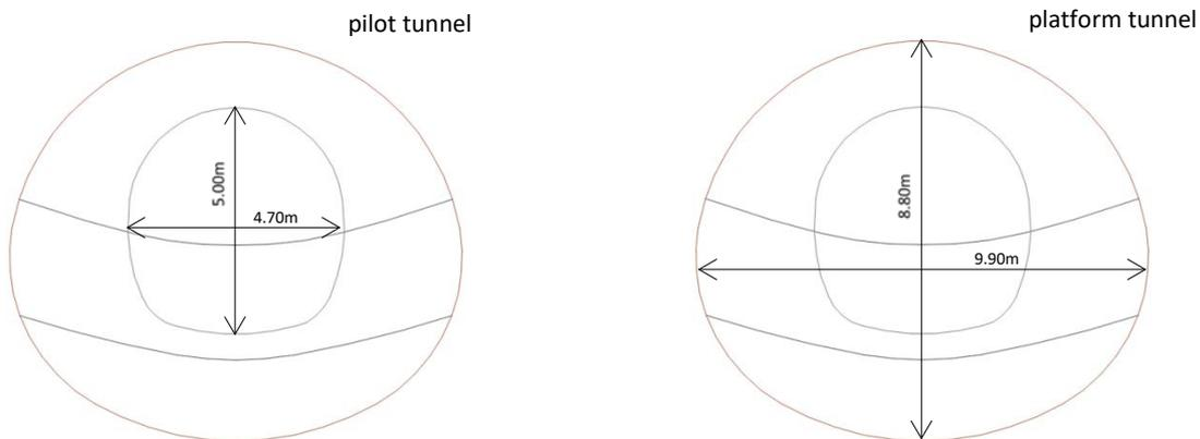
Figure 39: Dimensions of sections of interest
