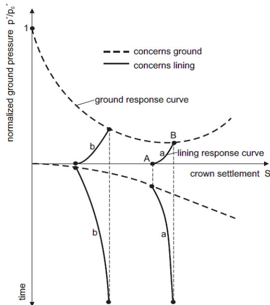
Figure 8: Relationship of ground pressure and timing of support installation after Pacher (1964)
