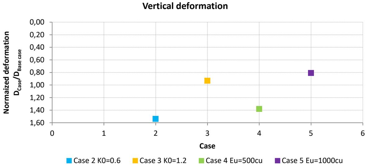
Figure 43: Normalized vertical deformations (crown) of different cases
