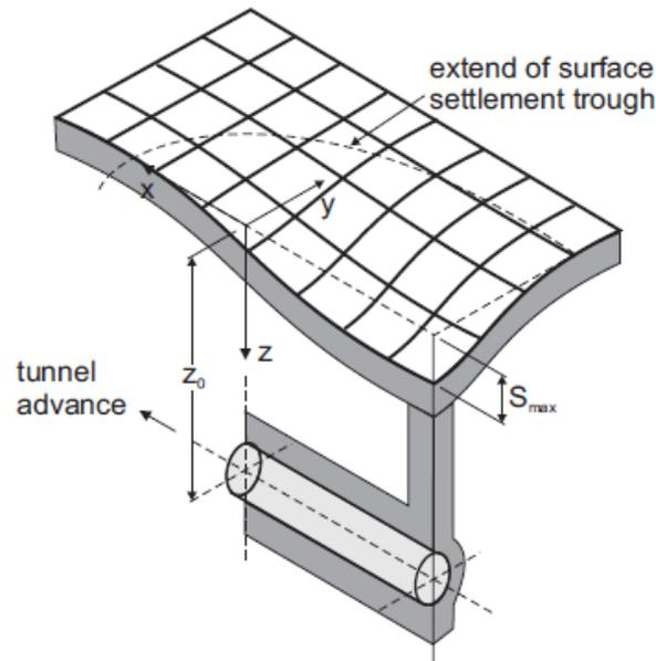
Figure 13: Three dimensional induced settlement trough (Attewell, 1986)
