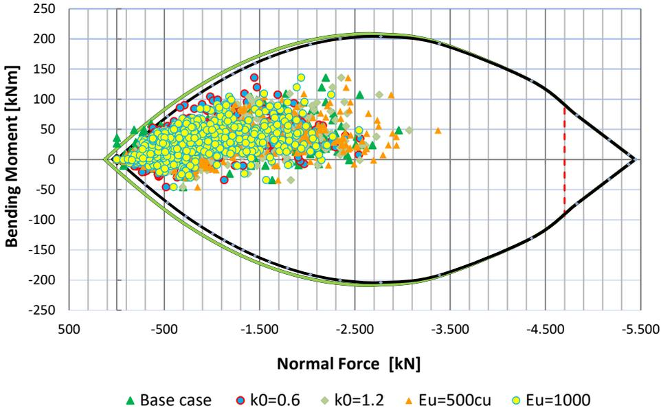
Figure 57: Bending moment vs. normal forces – All cases platform tunnel 3D (Nasekhan, 2016)
