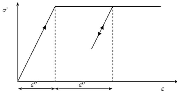
Figure 34: Main principle of linear elastic perfectly plastic model
