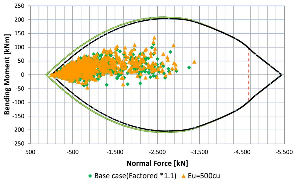
Figure 59: Bending moment vs. normal forces – base case vs. worst case 3D (Nasekhian, 2016)
