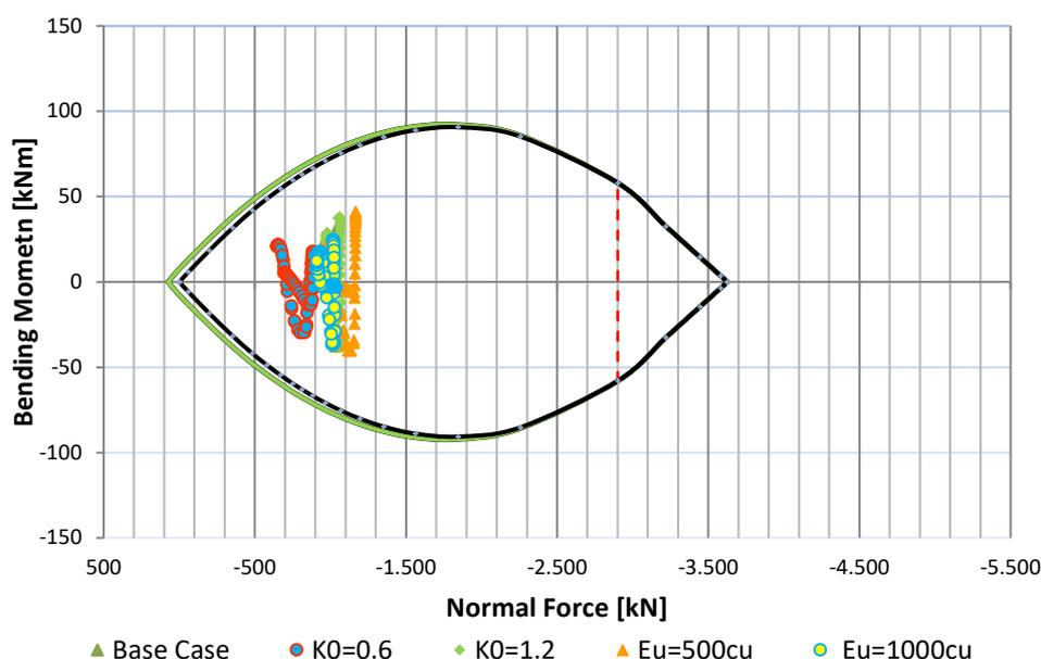
Figure 45: Bending moment vs. normal forces – All cases pilot tunnel
