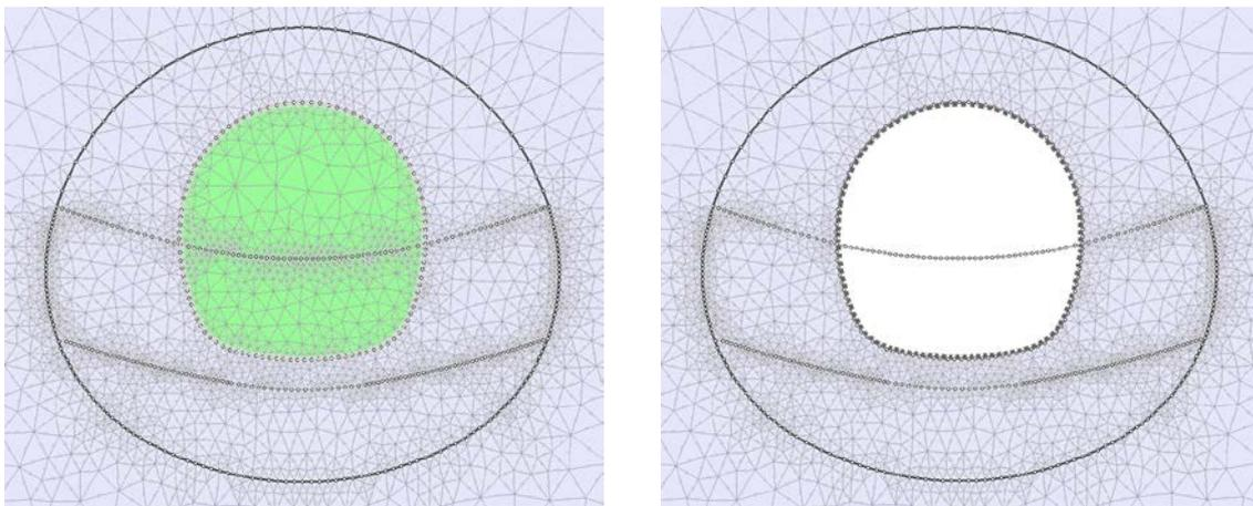
Figure 42: Excavation sequence pilot tunnel
