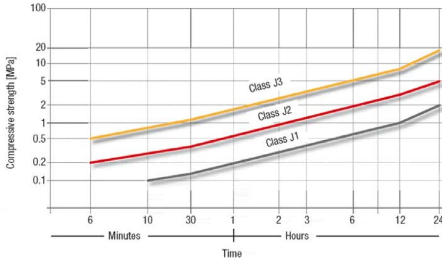
Figure 9: Early age strength development of sprayed concrete (Sika, 2012)
