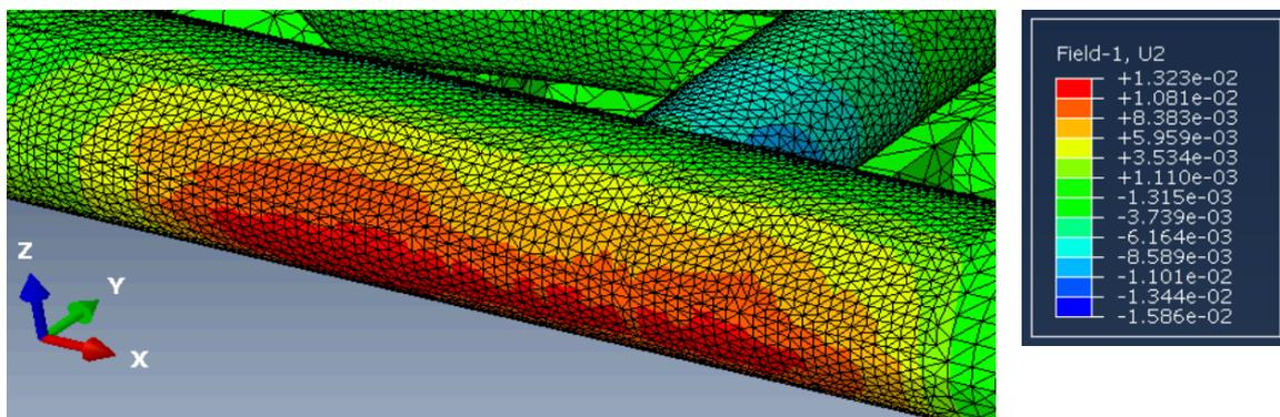
Figure 49: Horizontal deformations platform tunnel base case
