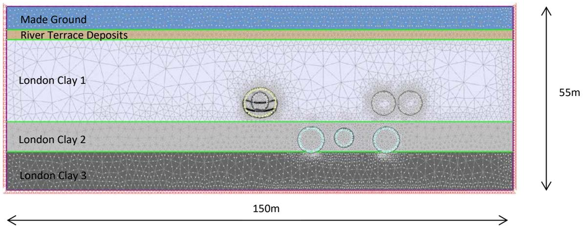
Figure 32: 2D section with existing assets and new SCL tunnel
