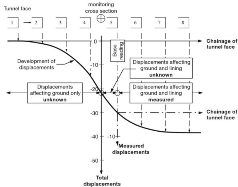
Figure 14: Displacement development ahead of the tunnel face (Stärk, 2009)
