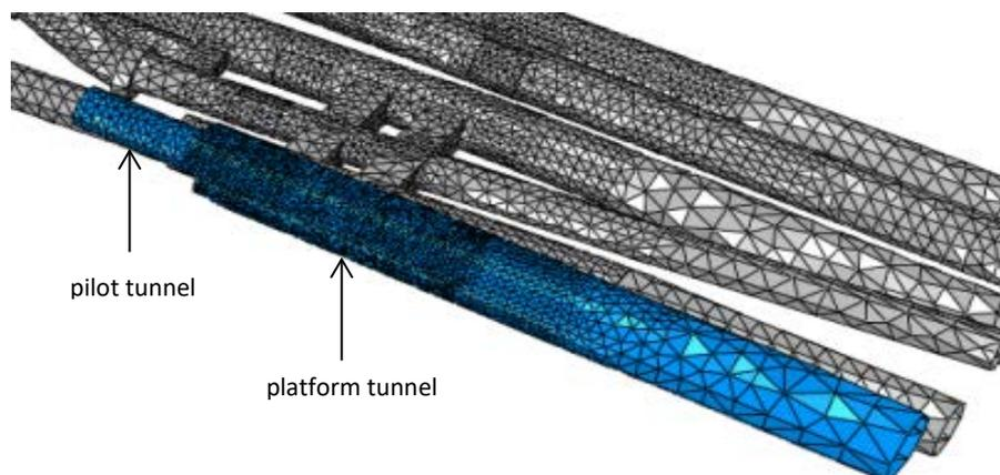
Figure 26: FE model of pilot tunnel and platform tunnel enlargement
