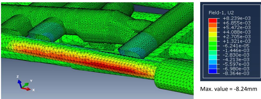
Figure 41: Horizontal deformations pilot tunnel Base Case
