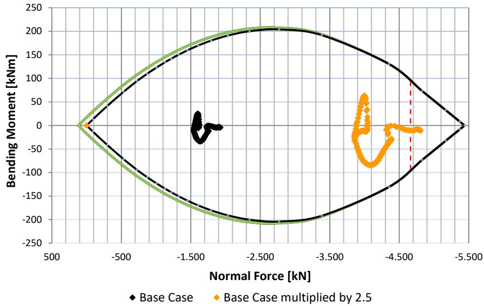
Figure 60: Bending moment vs. normal forces – base case factored by 2.5 2D
