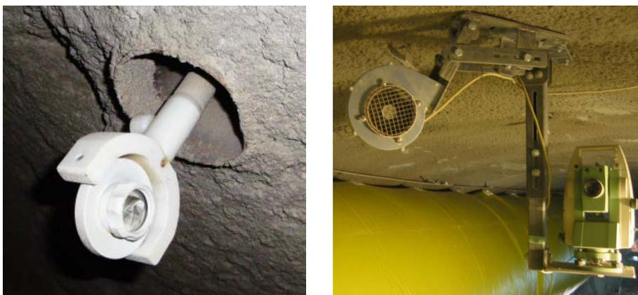
Figure 16: Installed reflector pin left, installed robotic station right (ÖGG, 2014)
