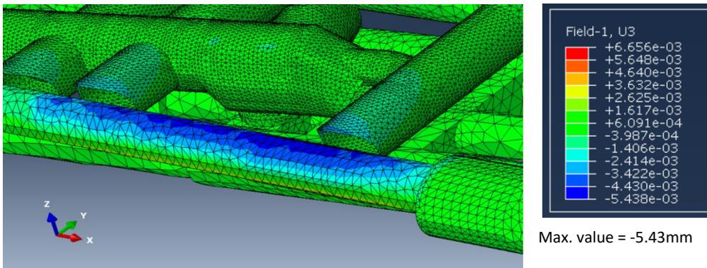
Figure 40: Vertical deformations pilot tunnel Base Case
