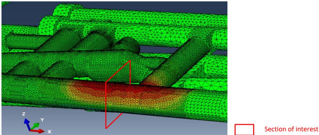
Figure 38: Section of interest in the 3D model
