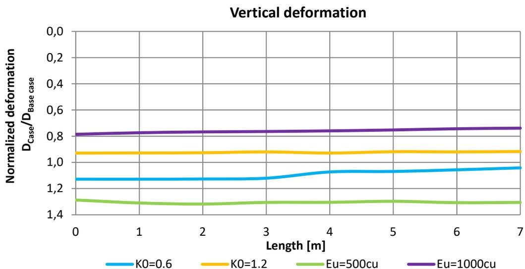
Figure 53: Normalized vertical deformations (crown) of different cases 3D (Nasekhian, 2016)
