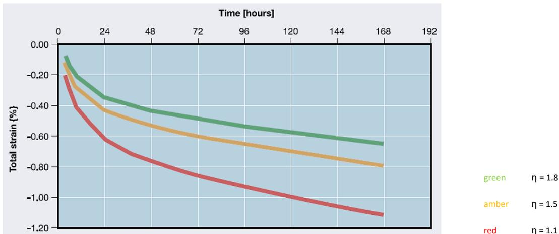
Figure 21: Strain paths corresponding to safety levels  $\eta$  (Jäger, 2005)
