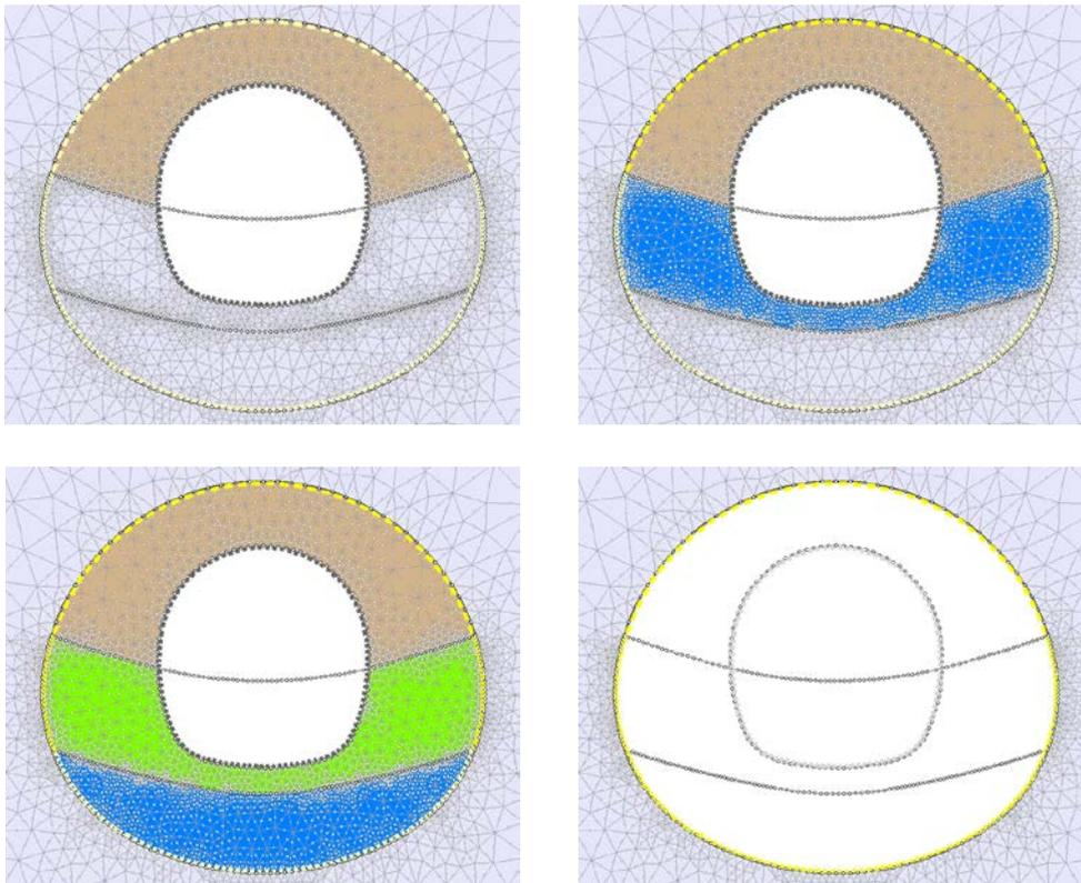
Figure 50: Excavation sequence platform tunnel
