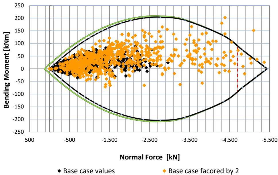
Figure 61: Bending moment vs. normal forces – base case factored by 2.0 3D (Nasekhian, 2016)
