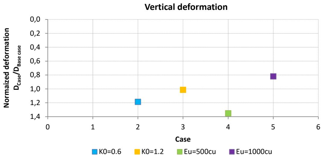
Figure 52: Normalized vertical deformations (crown) of different cases 2D
