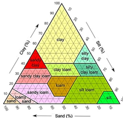
Figure 1: Soil types by clay, silt and sand composition (USDA)
