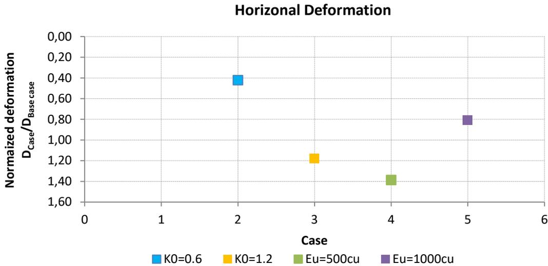
Figure 54: Normalized horizontal deformations (sidewall) of different cases 2D
