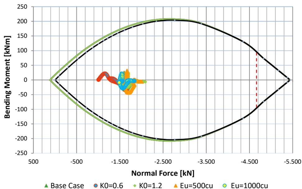
Figure 56: Bending moment vs. normal forces – All cases platform tunnel 2D
