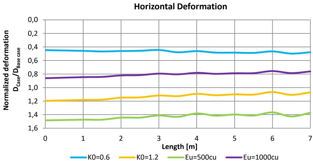
Figure 55: Normalized horizontal deformations (sidewall) of different cases 3D (Nasekhian, 2016)
