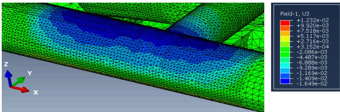
Figure 48: Vertical deformations platform tunnel base case
