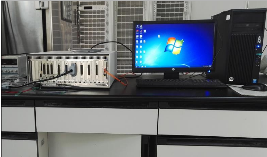
Figure 6-22; Real-time simulator (left) and the Host PC (right)
