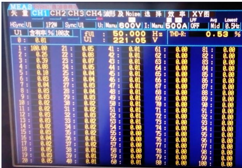
Figure 6-8; THD of the output voltage in 50 Hz, K_{IP} = 4.9 , screenshot of power analyzer
