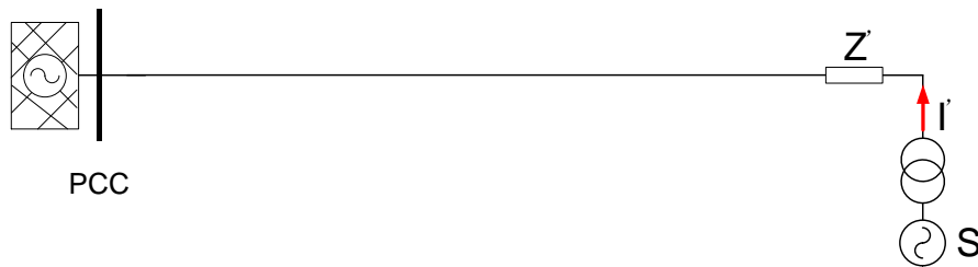
Figure 4-28; Equivalent simplification of the collection system
