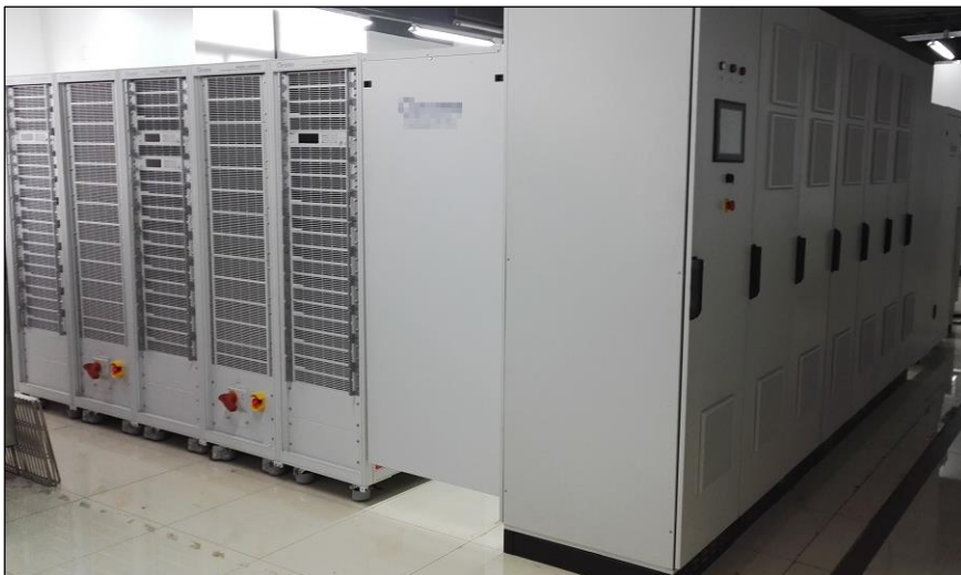
Figure 6-22; Real-time simulator (left) and the Host PC (right)
