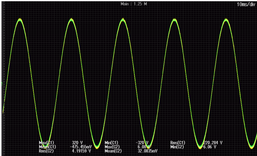
Figure 6-7; Output vs. reference voltage in 50 Hz, K_{IP} = 4.9 , screenshot of oscilloscope
