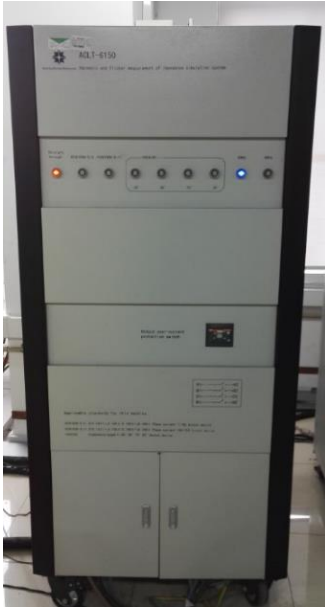
Figure 6-47; Photo of the impedance cabinet
