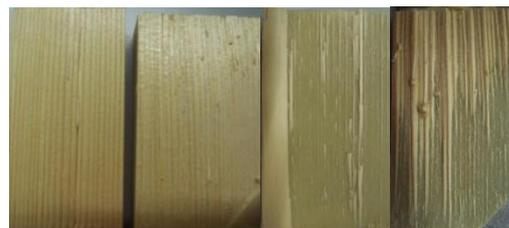
S-PU-G-03  $F_{\max} = 50,83 \text{ kN}$
