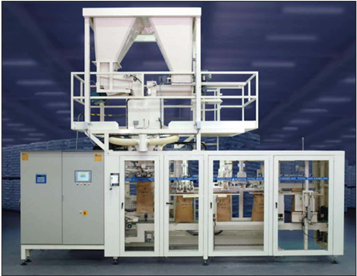
Figure 41: Arodo Automatic Bagging Line 408
