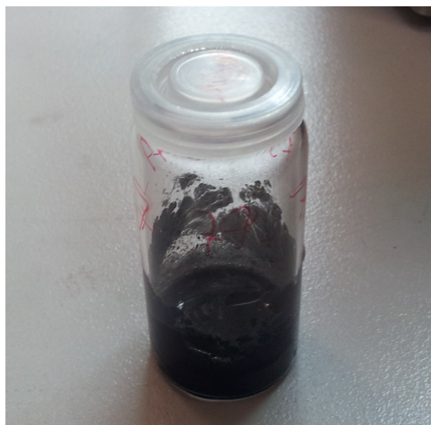
Figure 3.4: Dispersion solution of a catalyst prepared on a GDE sheet with water added.
