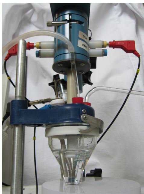
Figure 3.3: Cyclic voltammetry 3-electrode set-up with gas inlets.
