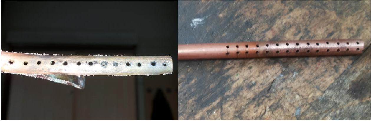
Figure 3-9: Distribution pipe at the evaporator inlet before (left) and after the modifications (right)
