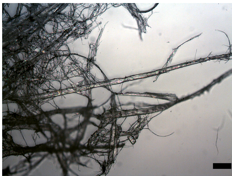
Figure 4.7 Unbeaten PGW pulp fibres without primary fines (Norske_0023) Magnification: 10x, Bar at bottom right = 100 \mu\text{m}
