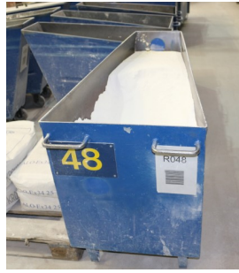
Figure 3-3: Single container for carousels
