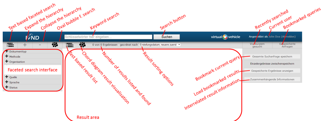
Figure 5.1.: The landing page of the information cockpit, the proof of concept implementation. Annotations describe the components.
