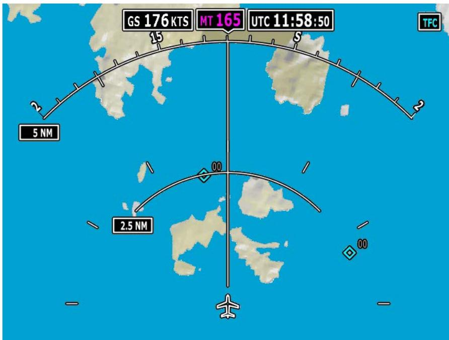
Figure 3.1: Example image of the moving map displayed in the cockpit. In accordance with TCAS-symbolism, the position of traffic on the map is indicated by a diamond and the relative altitude is shown as a 2-digit number [48].
