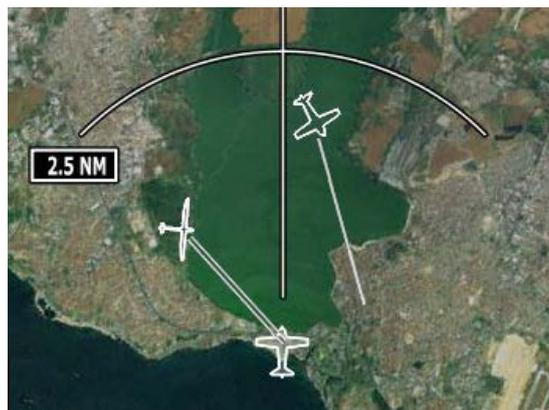
(e) Display variant E. The full implementation of the proposed display concept in section 4.2: Oriented aircraft symbols with relative track & priority line (here: glider from left has priority, small aeroplane ahead).
