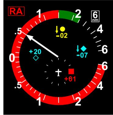
Whereas in commercial aviation TCAS I and II represent the standard cockpit equipment for airborne collision avoidance, the introduction of a similar system for use in uncontrolled airspace and visual flight has only just begun. For use under VFR, current proprietary solutions acquire and display the position of other aircraft (Table 2.2). They also provide aural and visual traffic advisories in the form of alerts.
