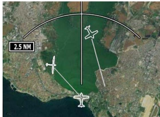
(d) Display variant D: Oriented aircraft symbols with relative trackline (here: glider from left on a predicted collision course with the ownship, small aeroplane ahead). The relative line shows if traffic is on collision course or not.
