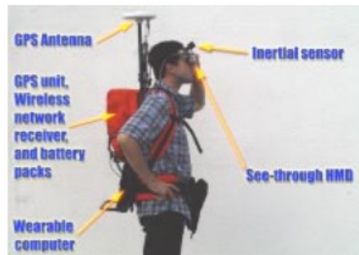
Figure 3.15: Battlefield AR system (BARS) developed in 2000, taken from Yohan et al. (2000)
