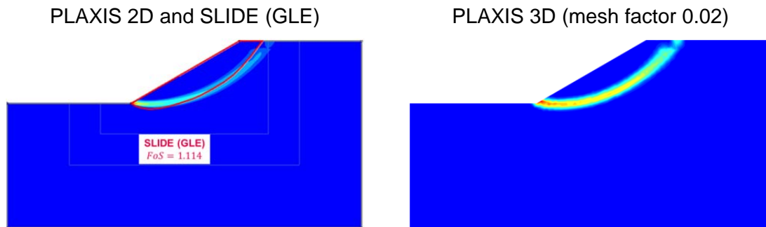
Figure 51 Comparison failure mechanisms of the unsupported slope (2D vs. 3D)
