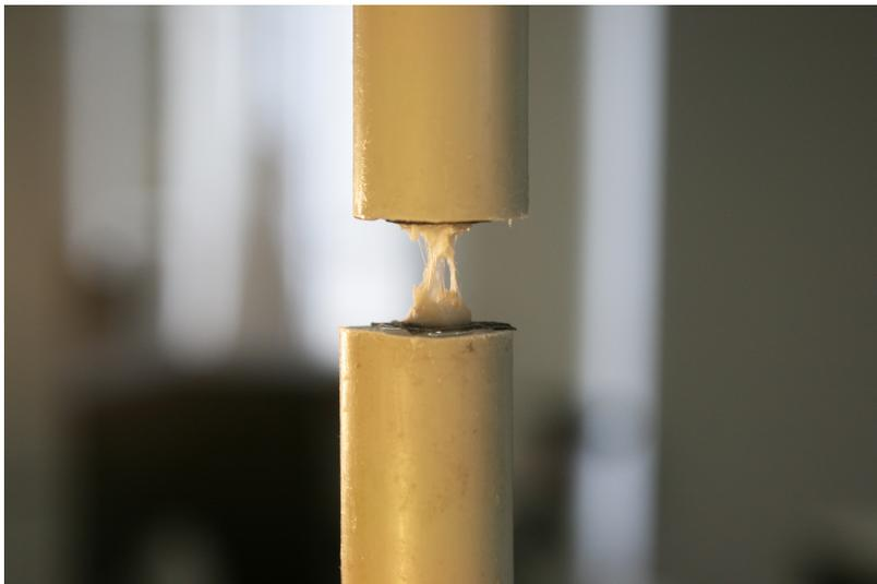
Figure 2.10: Example illustration of the end stage of a successful direct tension test.
