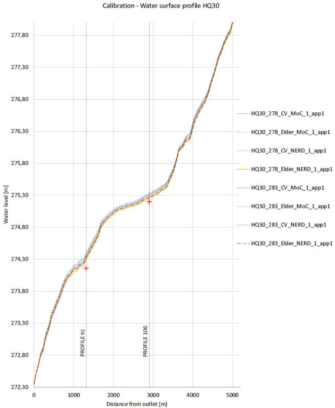
Figure 41 Calibration - HQ30 - Water surface profile
