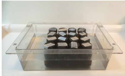
Figure 2.12: Phantom consisting of 16 glass bottles filled with Gadovist-doped water of different concentrations.
