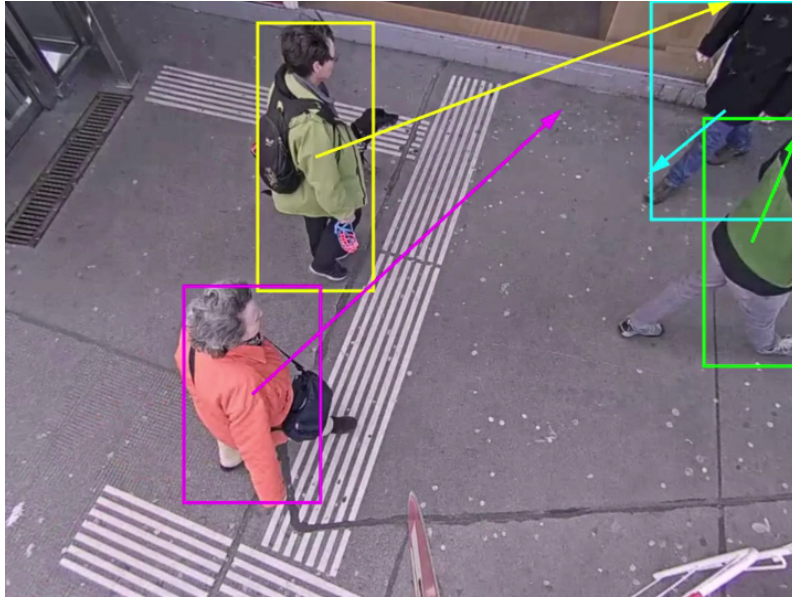
Figure 1.1: Illustration of pedestrian intent prediction. The coloured boxes correspond to pedestrian detections. The arrows indicate the intended destination estimated by the system based on the information of consecutive frames.
