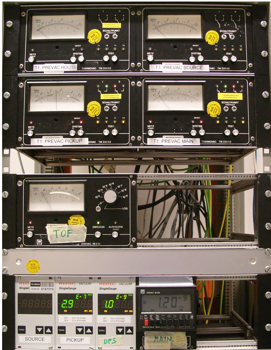
Figure A.9.: Vacuum pressure monitors. Although the TM 220 S 2 model can control 2 pirani gauges, there is one separate monitor for every single prevacuum-line. Every monitor is labeled with respect to the position of its associated measurement gauge.
