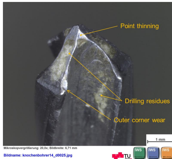
Fig. 66: Tip of a discarded three-flute surgical drill bit (Synthes 324.213, \varnothing 4.3 mm)
