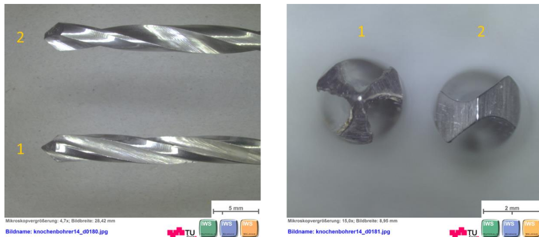
Fig. 33: Comparison of two- and three-flute surgical drill bits 11
