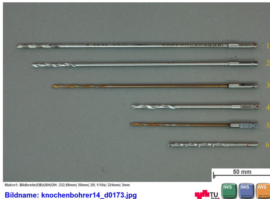
Fig. 5: Different types of surgical drill bits 1: Synthes 315.33 1 , \varnothing 3.2 mm; 2: Synthes 310.290 1 , \varnothing 3.2 mm 3: Synthes 310.23 1 , \varnothing 2.5 mm; 4: Synthes 310.350, \varnothing 3.5 mm (new) 5: Synthes 310.25 2 , \varnothing 2.5 mm, 6: manufacturer unknown 2 , \varnothing 3.2 mm
