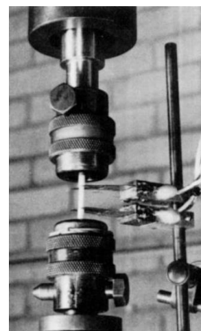
Fig. 9: The clamping of the testing machine with the extensometer in position (Dickenson et al. 1981)
