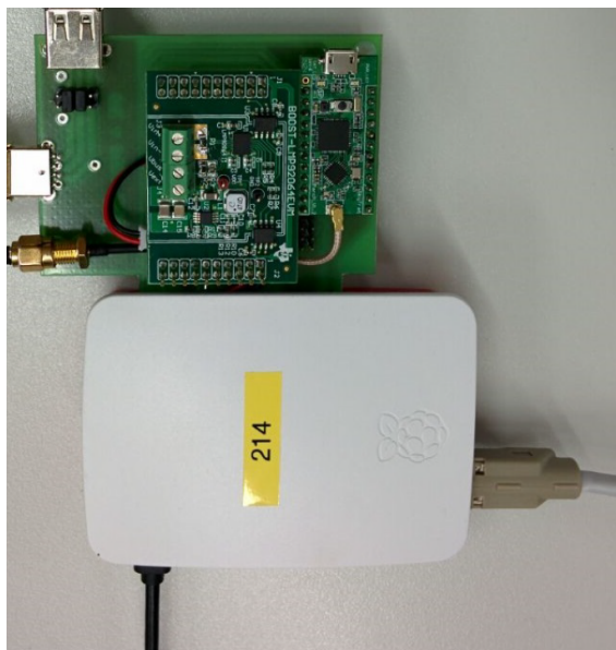
Figure 5.8: Energy measurement setup consisting of a Raspberry Pi 2 model B connected to a TI LMP 92064.
