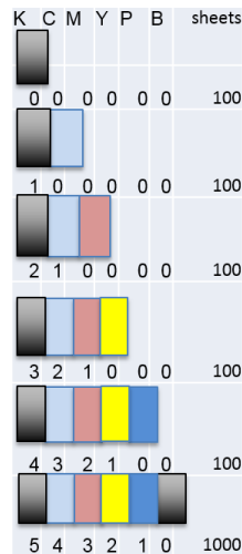
Figure 6.1 Print trial A. The stack of printed sheets obtained from the trial. The numbers below the colours represent the amount of back-traps of one colour.
